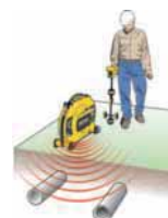
Induce a signal to locate utilities
